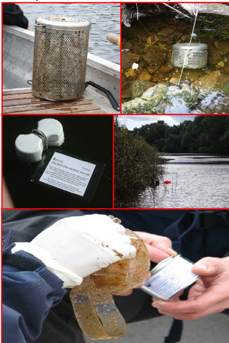
Figure 3.8 Upper left: Metal canister containing the POCIS and SPMD sampler. Upper right: Deployed metal canister. Middle left: Buoy keeping the deployed metal canister floating below the water surface with a floating pamphlet describing the sampling and why it should not be removed. Middle right: Buoy keeping the deployed metal canister floating below the water surface. Lower: SPMD membrane removed from spindle holder after the sampling period and being transferred to a clean transport container.
