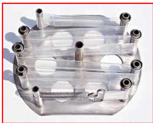
Figure 3.4 Spider carrier with mounted lipid filled membrane for SPMD sampling.
