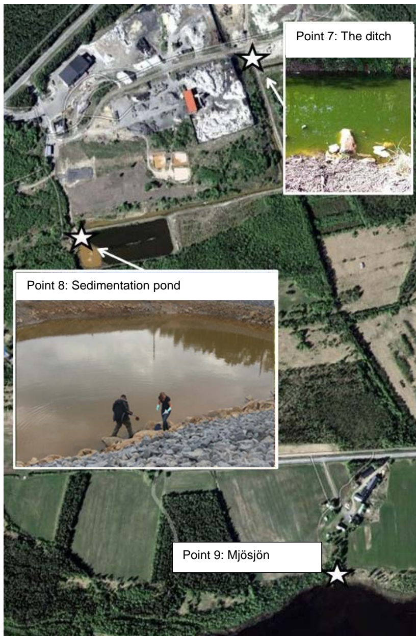
Figure 3. Three samples were taken at Brännkläppen landfill, of which two were within the landfill site and one in Mjösjön, the receiving water for leachate from the landfill.
