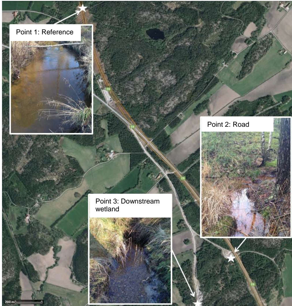
Figure 1. Samples were taken at three points, to investigate leaching and spread of concrete additives from the road construction. Point 1 is a reference point upstream that has not been affected by the recycled concrete. Point 2 was selected to be as close to the recycled concrete as possible. Point 3 was located approx. 300m from the concrete road construction.
